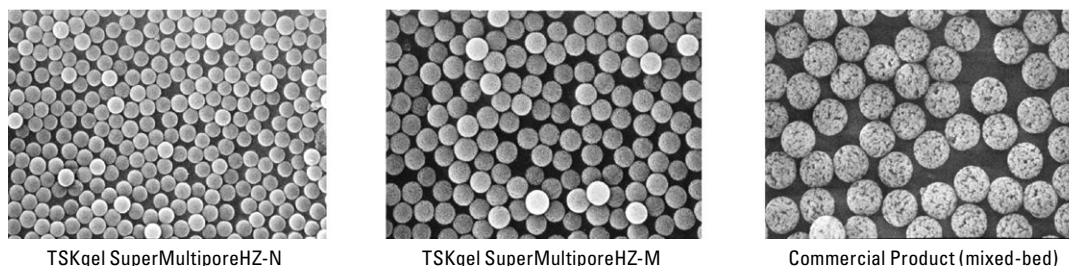
Figure 18: TSKgel SuperMultiporeHZ columns are packed with monodisperse particles
