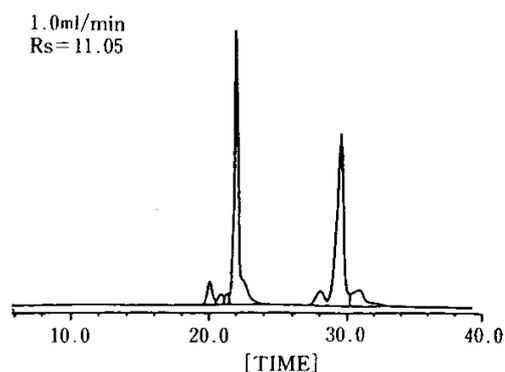
**Figure-6** Effect of flow rate on protein separation
