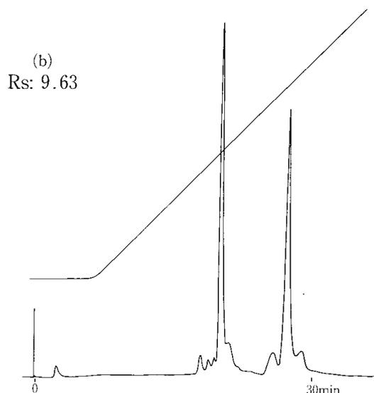
**Figure-1** Chemical stability in TSKgel SuperQ-5PW (CIP washing with 0.5N NaOH)
