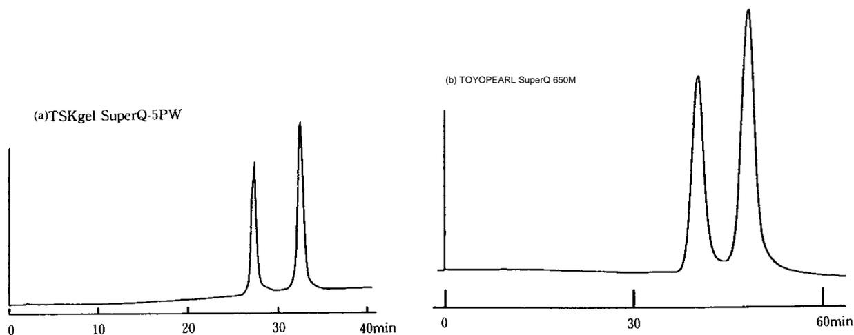
**Figure-18** Scale up from TSKgel SuperQ-5PW to TOYOPEARL SuperQ 650M (4)
