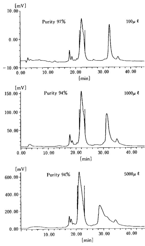
**Figure-10 Separation of mouse monoclonal antibody A (IgG<sub>1</sub>)**
