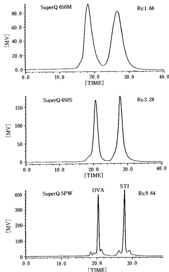
**Figure-15** Scale up from TSKgel SuperQ-5PW to TOYOPEARL SuperQ 650S (1)
