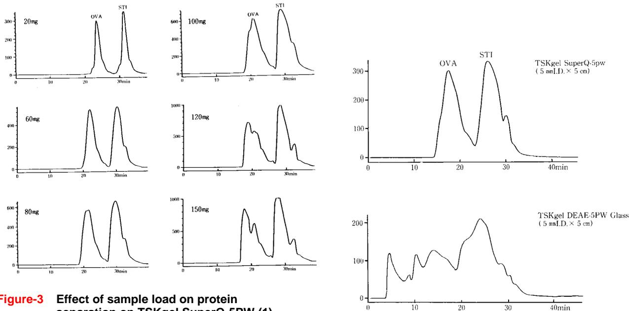
**Figure-3** Effect of sample load on protein separation on TSKgel SuperQ-5PW (1)
